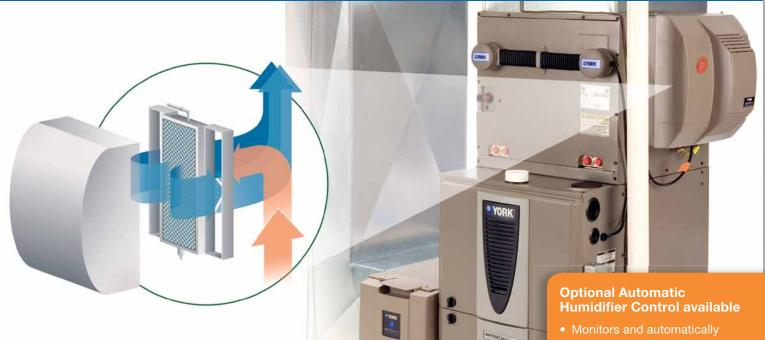
Affinity™ Whole-Home Humidifiers use a natural evaporation process to generate comfortable humidity. Water flows through an evaporative pad and warm air from the furnace is drawn through it. This creates the pure water vapor that your HVAC system circulates throughout your home for optimum comfort.
